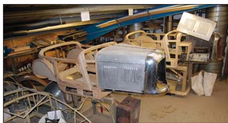
WOODWORK SHOP; Two original Austin 7 Swallows under construction and a de Portago car.
